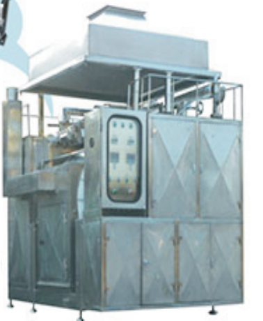
★ SF105-3 蟹味棒烤機 ROASTER SIZE: L2200 x B2700 x H4000 POWER: 2.57kw WEIGHT: 5200kg 轉鼓直徑: φ1500
