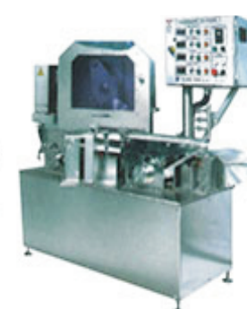
★ SF111圓盤斜切機 DIAGONAL CUTTER SIZE: L1200 x B750 x H1700 POWER: 0.9kw WEIGHT: 300kg
